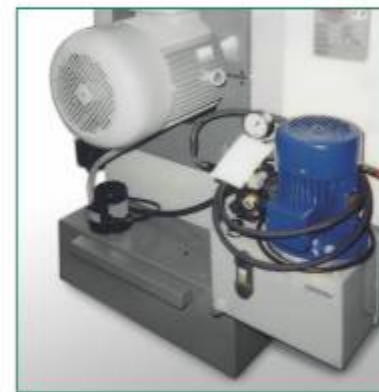
Vasca refrigerante Coolant tank
