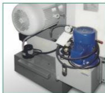
Vasca refrigerante Coolant tank
